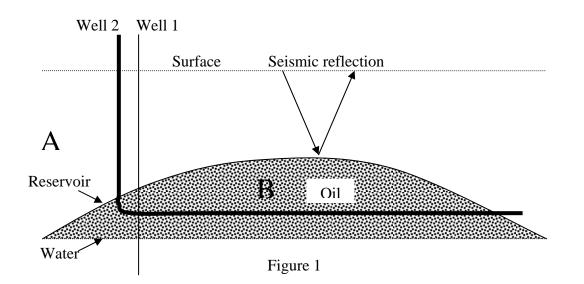
In the past, this was not a huge problem because most wells were drilled nominally vertically though the reservoir like Well 1. New improvements in drilling technology enable more complex wells that can be horizontal like Well 2. These wells can be much more efficient since they have much more surface area contact with the reservoir.
