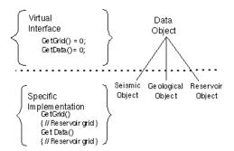
Any object derived from a Data Object can feed data to an object derived from a Grid Object, see figure 4b. This allows objects to be mixed and matched within applications providing the programmer with the building blocks to create integrated viewers. This process is simplified by the fact that all Data Objects are self contained and communicate through a well-defined interface.
